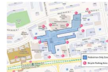
Pedestrian-only Zone (POZ) with bicycle parking outside the zone and POZ markings. Source: LTA
