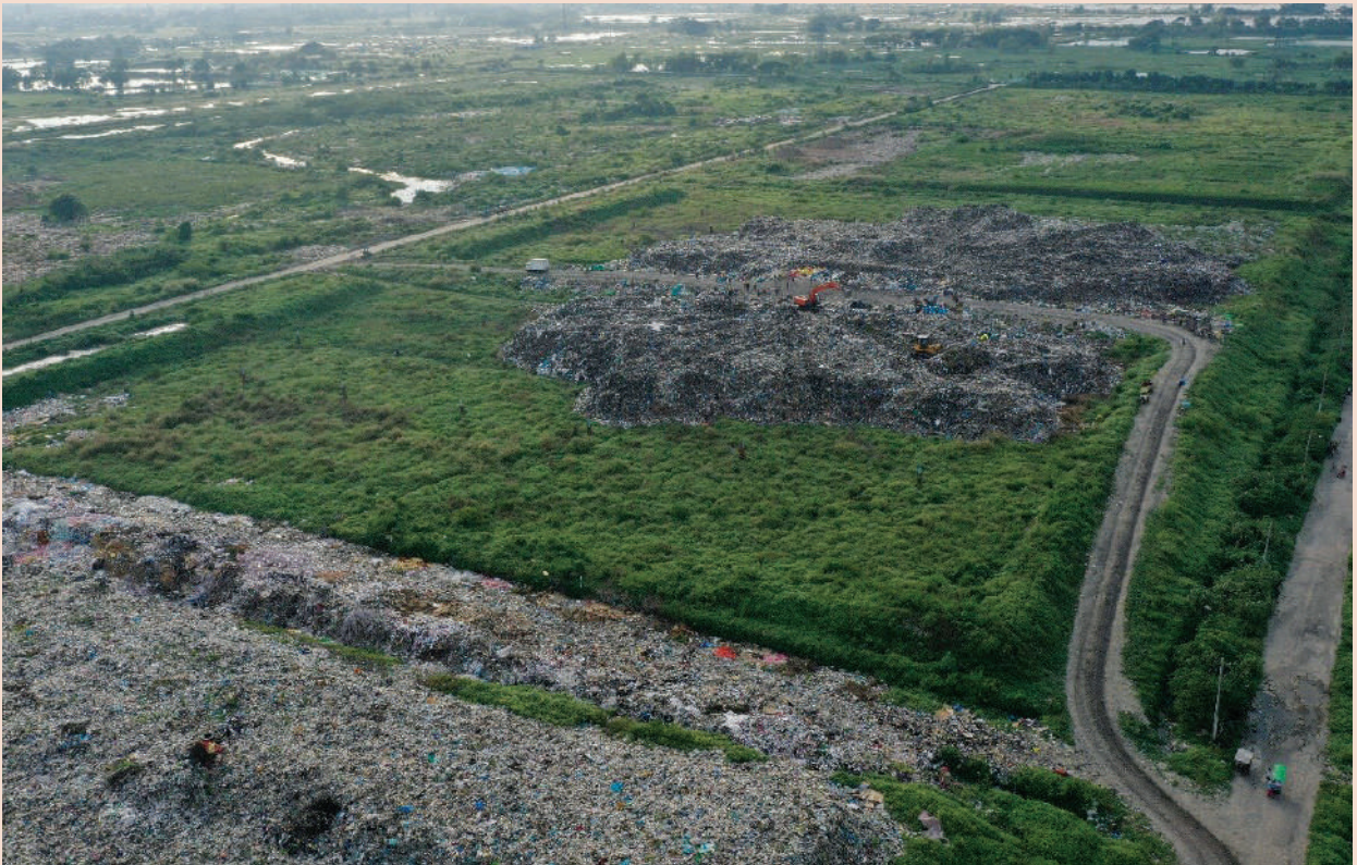
Through the Fukuoka method, the landfill site has been rapidly stabilised, and vegetation has begun to return. Image: Fukuoka City
