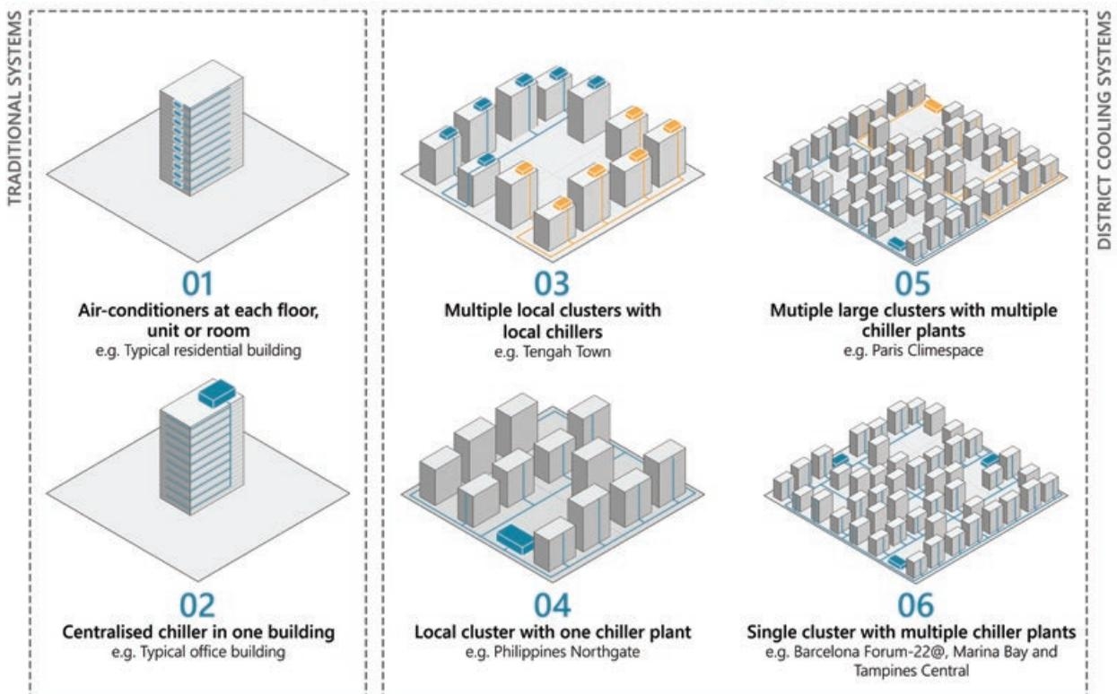
Figure 1. Typologies of active cooling systems.
